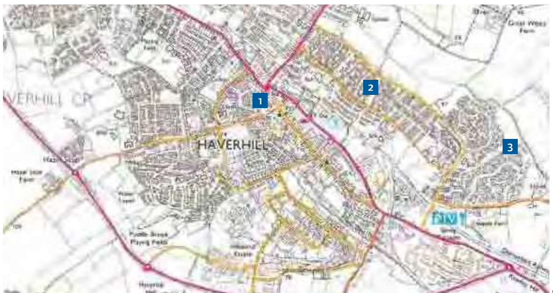
Figure 4.5 The plans of many UK villages, towns and cities illustrate different patterns of development over time, from (1) historic cores, through to (2) experimental 'Radburn' layouts from the 1960s, to (3) recent cul-de-sac/DB32-type layouts.
